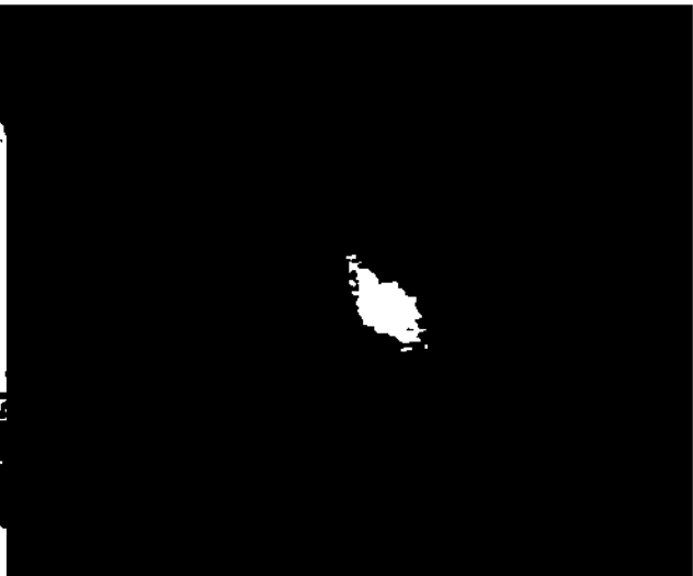
Figure 1.7. Photo of Center Spot Formation. The main beam observed is a direct path along the injector angle. Other faint light channels indicate beams for scattering of the central core region.
