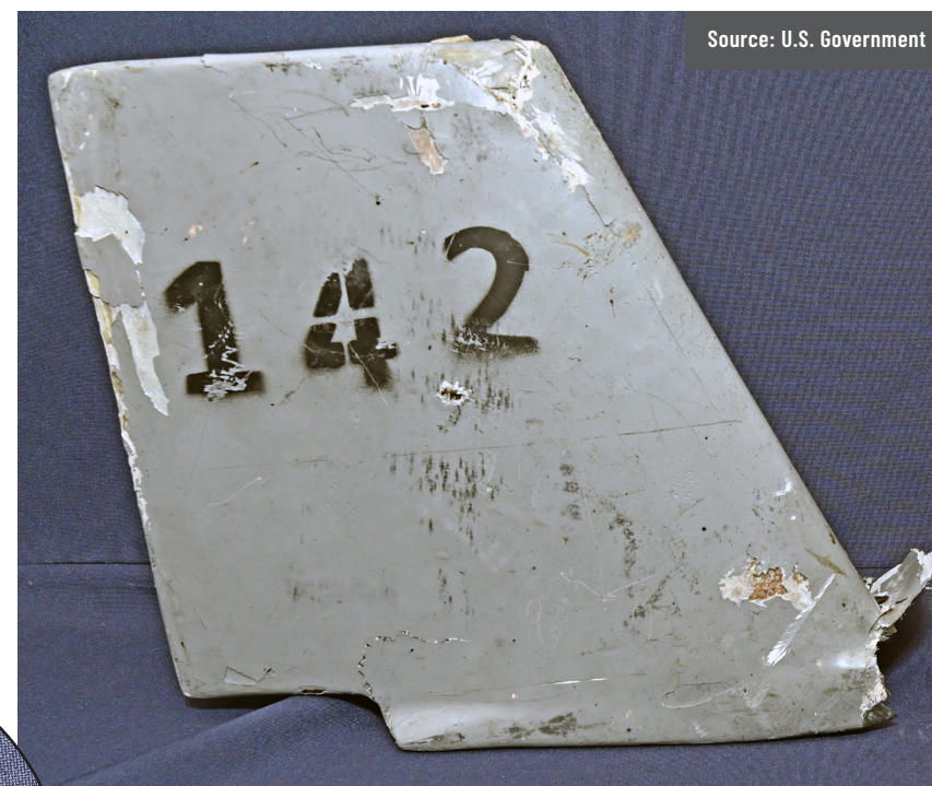
Shahed-131 wing stabilizer recovered from a 2022 attack in Iraq that Iran claimed
